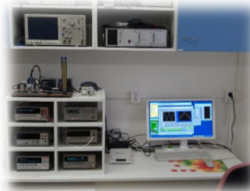
In-house developed systems for measurement of sensor properties, Electrometer Keithley 6517A and Keysight 34465A - precise measurement of high resistance materials with in-house fixtures with triaxial interconnection
