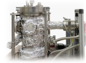
UHV - Deposition system combining two molecular evaporators and one boat evaporator, simultaneous deposition of various materials
