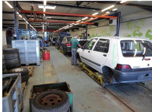
Renaults contributes to the collection and processing of the 25% of the total End-of-Life vehicles (ELVs) in France through **Indra, operating a network of 400 dismantlers** processing more than 95,000 vehicles in 2015.
