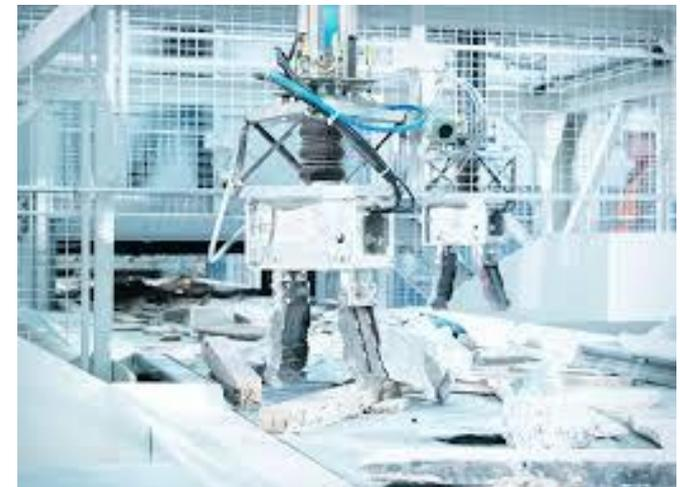
**Examples Zen Robotics:** Lukka, T.-J., Tossavainen, T., Kujala, J.-V., Raiko, T., 2014, ZenRobotics Recycler – Robotic Sorting using Machine Learning, Sensor Based Sorting.
