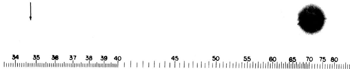
FIG. 1. A direct reproduction of the first plate in which there was an indication of second harmonic. The wavelength scale is in units of 100 Å. The arrow at 3472 Å indicates the small but dense image produced by the second harmonic. The image of the primary beam at 6943 Å is very large due to halation.
