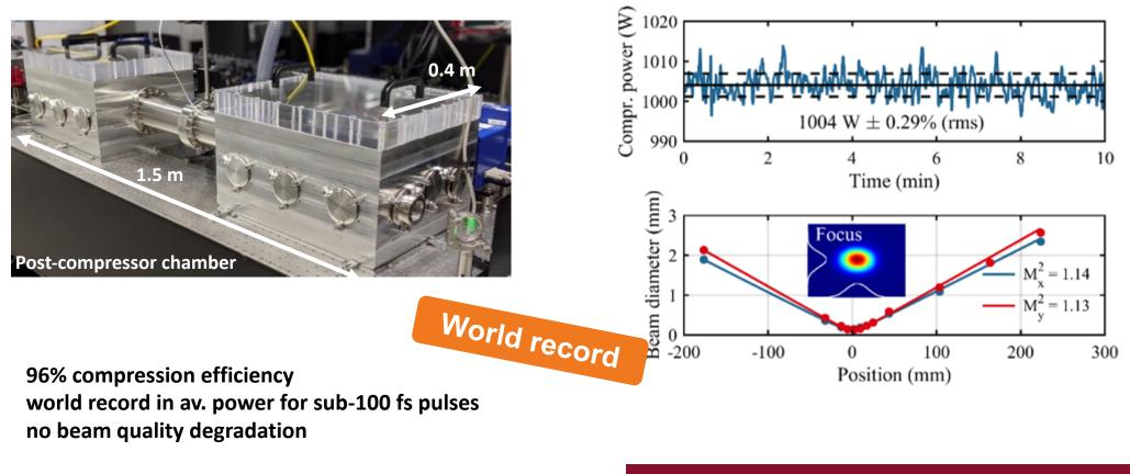
**31fs** pulses with **1mJ** pulse energy and **1kW** average power Investigation of few-cycle MPCs underwayHR1 and HR2-type parameters
