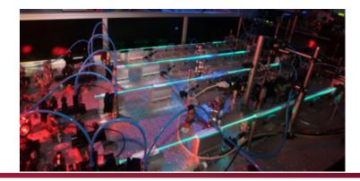
Nonlinear pulse compression down to few-cycle pulses
