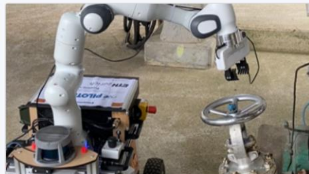
Autonomous hand-wheel valve detection and manipulation Autonomous detection and manipulation system of hand-wheel valves in
