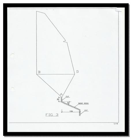
The mass of 30 000 tons and a horizontal force of 10 percent was applied at the rock center of gravity.
